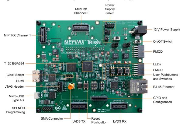
Figure 2: Trion® T120 BGA324 Development Board Components (Top)
