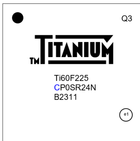
Figure 1 – Identifier for Device Manufactured using Substrate with Decoupling Capacitors
