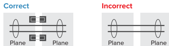
Figure 11: Use Stitching Capacitors across Split Planes
