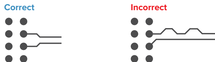
Figure 3: Route Differential Pairs Symmetrically and Always Keep Signals Parallel
