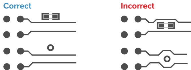
Figure 6: Do Not Place Components or Vias between Differential Pairs
