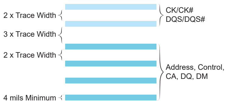
Figure 6: Trace Spacing Guidelines
