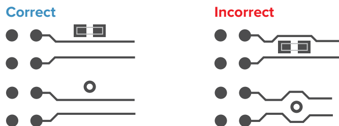
Figure 10: Do Not Place Components or Vias between Differential Pairs
