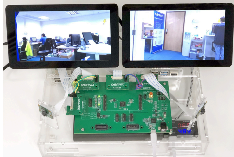
Figure 1: T20 Dual-Camera CSI-2 Example Design Setup (1)
