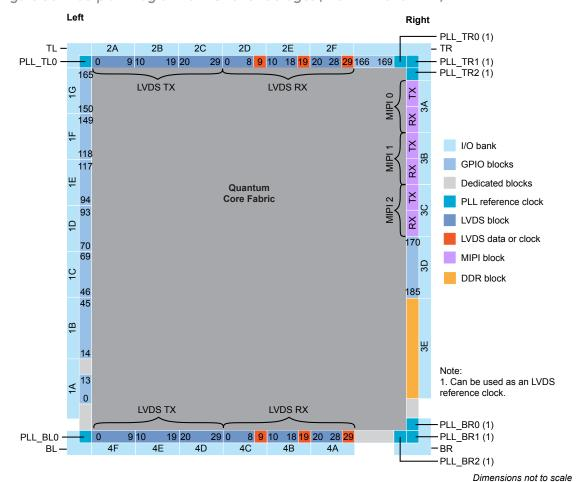
Figure 38: Floorplan Diagram for BGA576 Packages (with DDR and MIPI)
