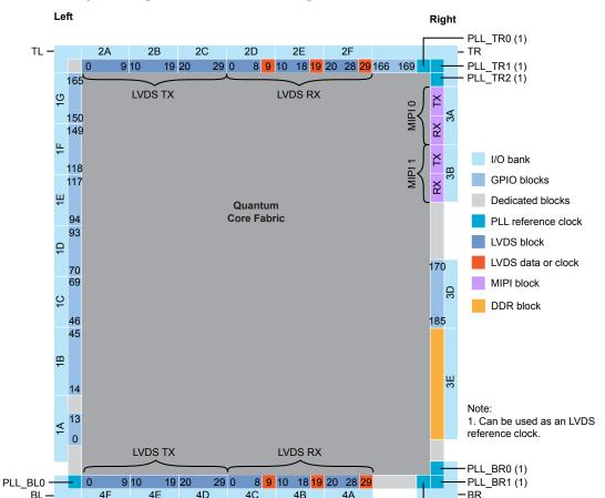
Figure 36: Floorplan Diagram for BGA324 Packages (with DDR and MIPI)
