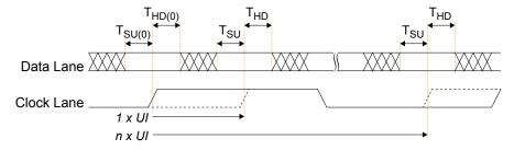
Figure 31: LVDS RX Timing (Edge-Aligned)
