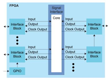
Figure 6: Interface Block and Core Connectivity
