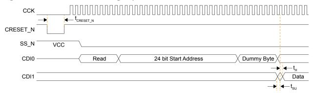
Figure 34: SPI Passive Mode (x1) Timing Sequence
