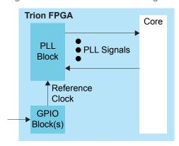
Table 13: PLL Signals (Interface to FPGA Fabric)
