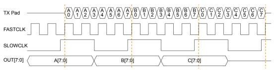
OUT is byte-aligned data passed from the core on the rising edge of SLOWCLK.
