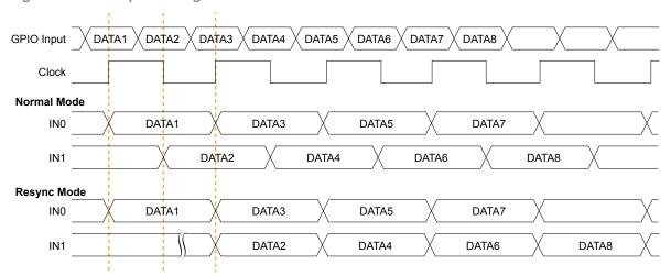
In resync mode, the IN1 data captured on the falling clock edge is delayed one half clock cycle. In the Interface Designer, IN0 is the HI pin name and IN1 is the LO pin name.
