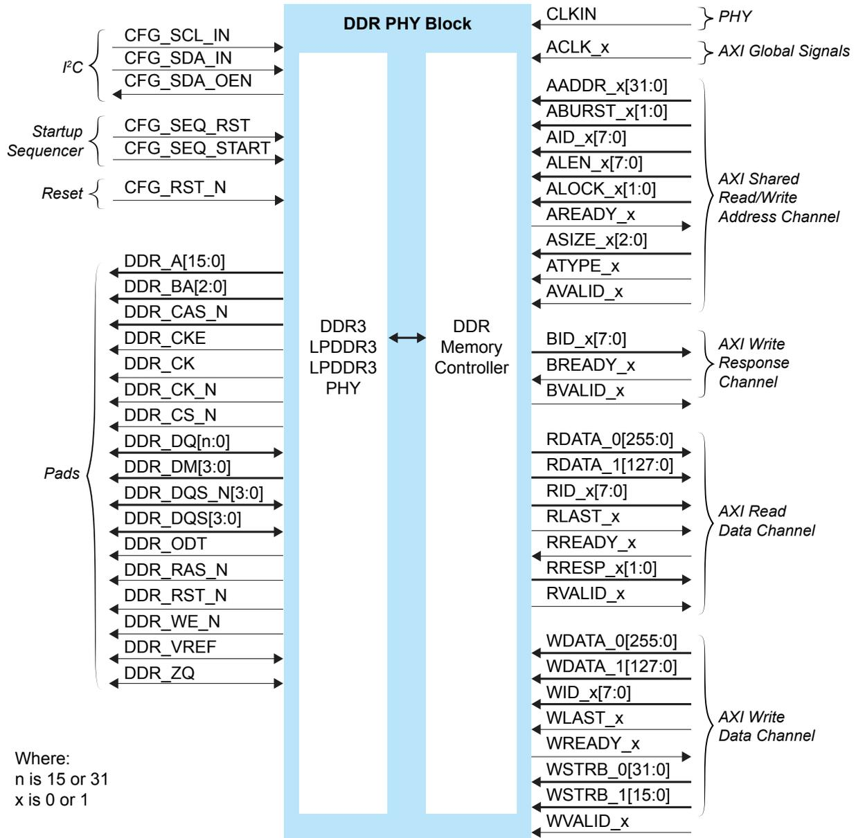
The DDR DRAM block supports an I<sup>2</sup>C calibration bus that can read/write the DDR configuration registers. You can use this bus to fine tune the DDR PHY for high performance.
