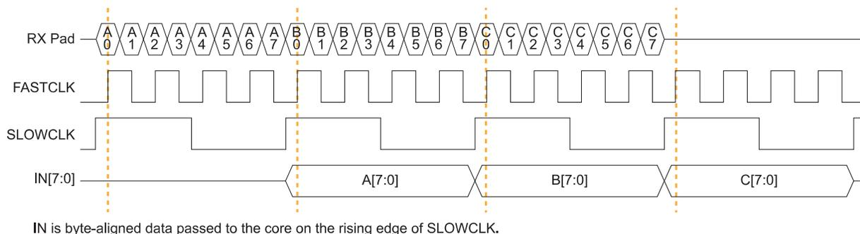
IN is byte-aligned data passed to the core on the rising edge of SLOWCLK.
