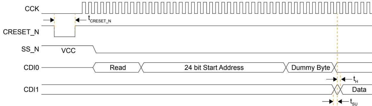
Figure 34: SPI Passive Mode (x1) Timing Sequence
