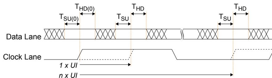
Figure 31: LVDS RX Timing (Edge-Aligned)
