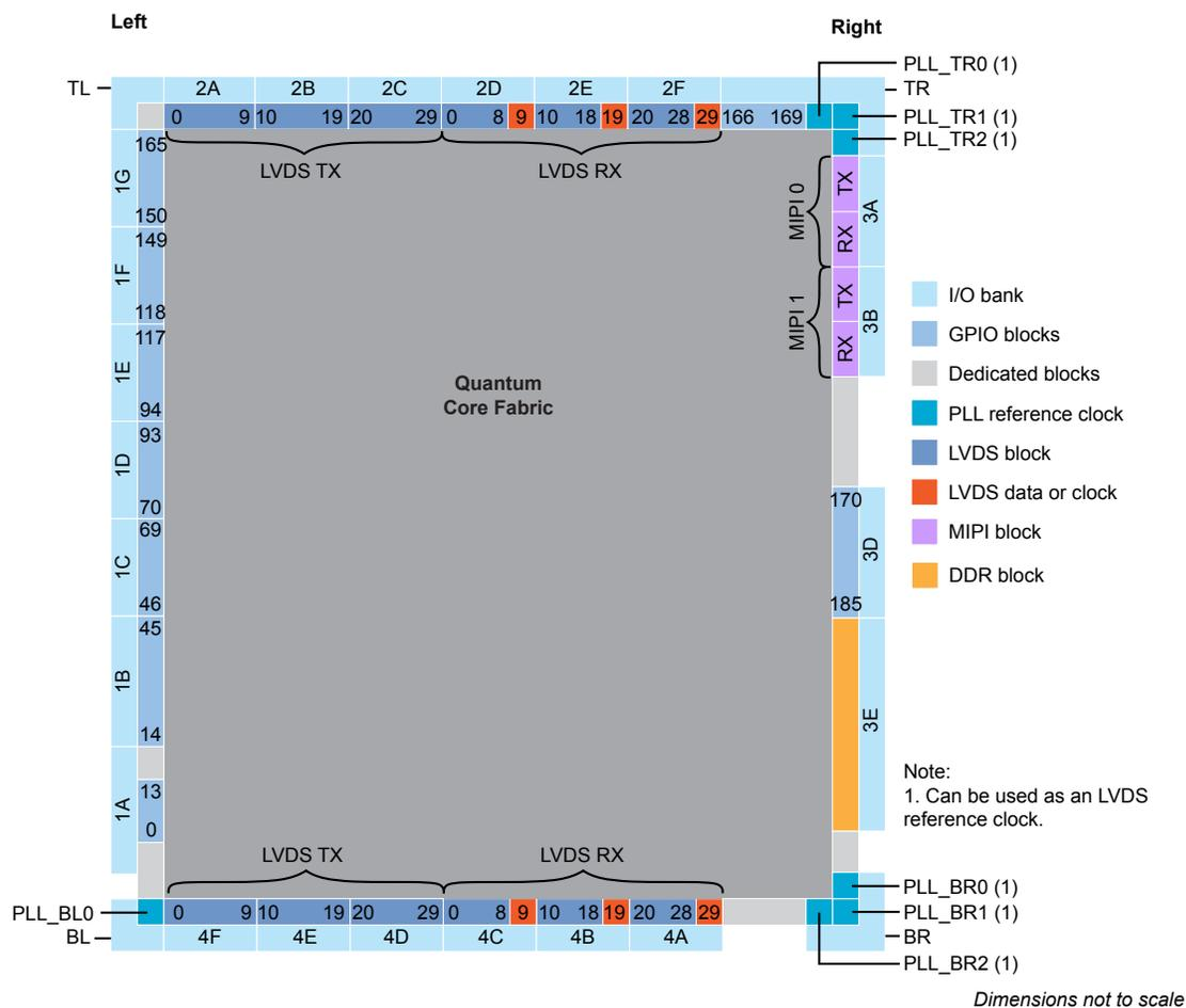
Figure 37: Floorplan Diagram for BGA484 Packages (with DDR)
