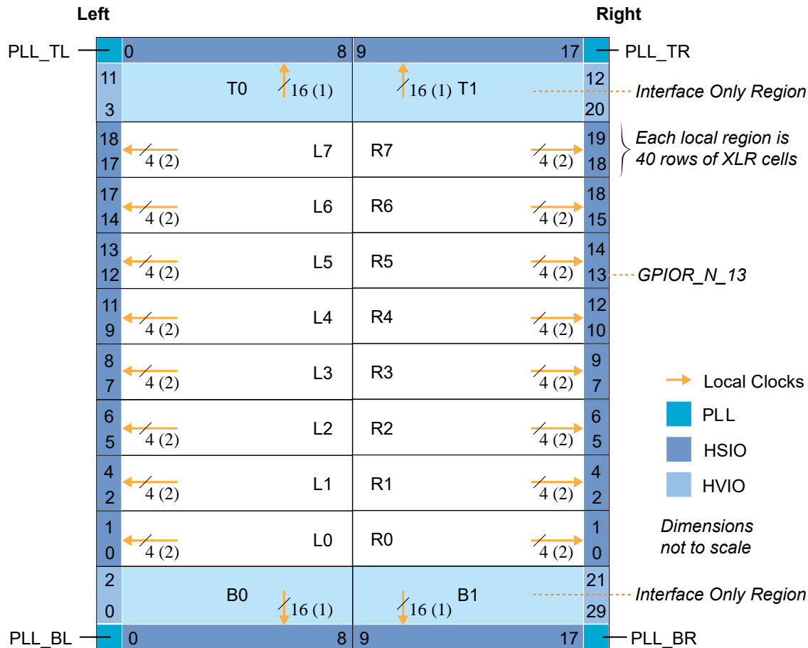
Figure 14: Clock Sources that Drive the Interfaces
