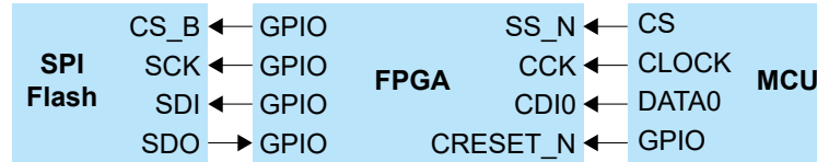
Figure 28: FPGA Configured with SPI Bus Connections to MCU and GPIO Emulated MCU SPI Bus Connections to SPI Flash
