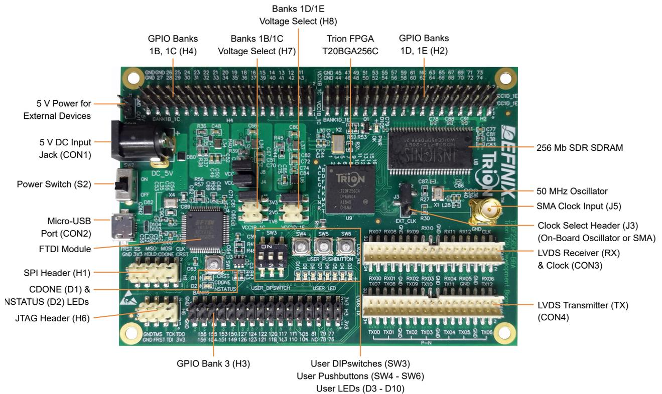
The FTDI FT2232H module has two channels to support SPI (FTDI interface 0) and JTAG (FTDI interface 1) configuration. It receives the T20 configuration bitstream from a USB host and writes to the on-board SPI NOR flash memory. After a reset in SPI passive mode, the FTDI controller can also write the configuration bitstream directly to the FPGA. Additionally, it supports direct JTAG programming mode in which it writes the configuration bitstream directly to the FPGA through the JTAG interface.
